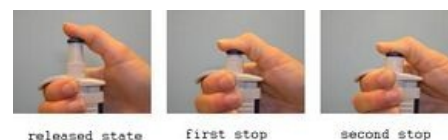
released state first stop second stop Pipetting positions
