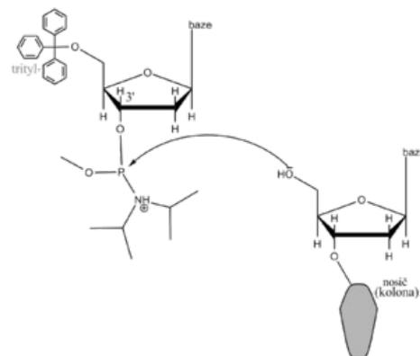
The phosphoramidite formula (5'-OH is blocked with trityl) and its binding to the growing polynucleotide, fixed to the support in the column.
