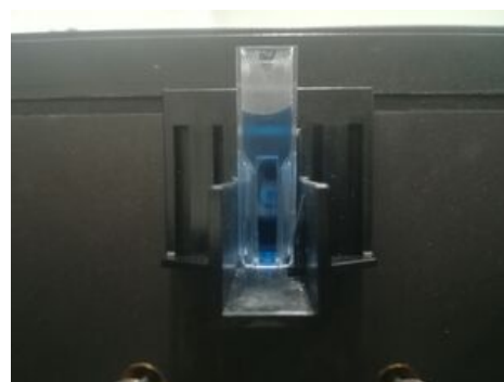
Inserted cuvette from the perspective of a passing beam.
