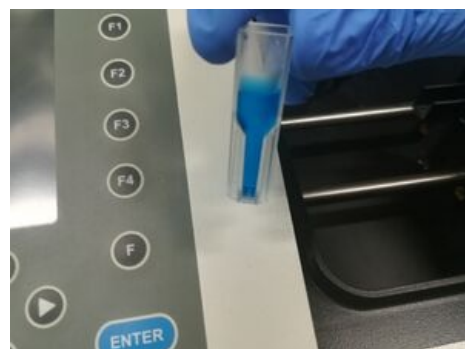
Narrowing of the cuvette in its lower part.
