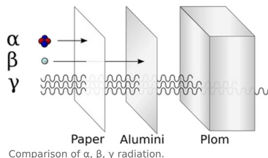
This barrier should be placed as close as possible to the source and serves us to reduce the intensity or to completely absorb the radiation.
