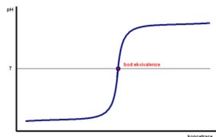
Graph of change in concentration and pH showing the equivalence point at pH=7
