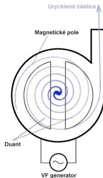
Scheme of the cyclotron
