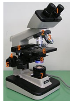
Parts of a Light Microscope: 1. Eyepiece (10X magnification) 2. Revolving objective head 3. Objectives 4. Coarse adjustment knob 5. Fine adjustment knob 6. Stage 7. Light Source 8. Condenser with diaphragm 9. Slide shift
