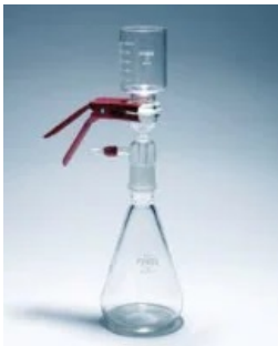
Vacuum filtration (picture from [2])
