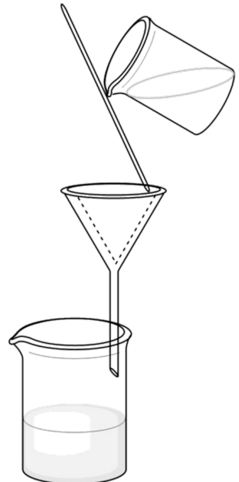
Filtration through a paper filter
