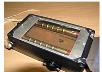
Ionization chambers in the dosimeter
