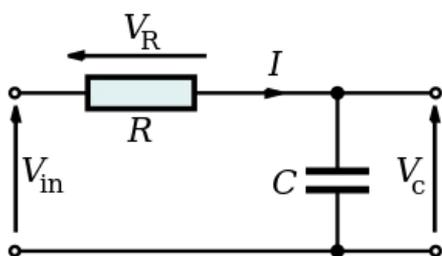
The transfer function of this filter is more complex because the ratio of the electrical resistance of the resistor and the capacitance of the capacitor does not change stepwise depending on the frequency. In addition, there is a phase shift. The transfer characteristics for amplitude and for phase are in the following figures:
