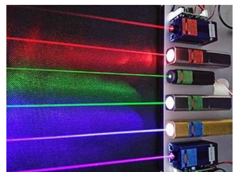
Six commercial lasers in operation, showing the range of different colored light beams that can be produced, from red to violet. From the top, the wavelengths of light are: 660nm, 635nm, 532nm, 520nm, 445nm, and 405nm. Manufactured by Q-line.
