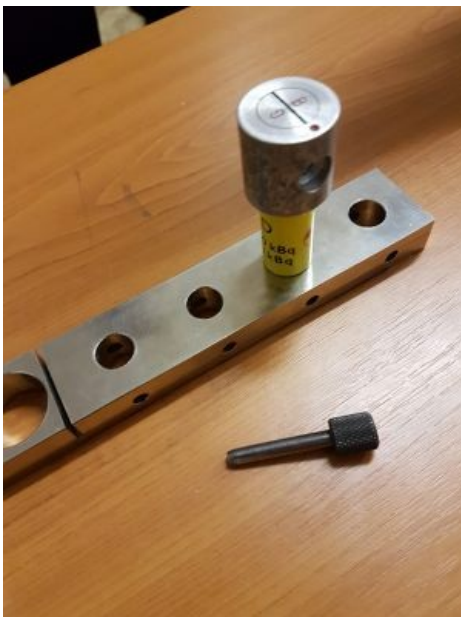
Radiation source in tripod holder and Arresting pin
