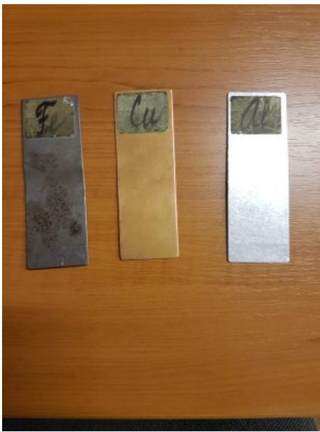
Absorbing plates: Iron(left) \ Copper(center) \ Aluminium(right)
