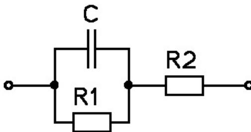
It is not complicated to express the dependence of the impedance of the model as a function of the resistance of both resistors, the capacity of the capacitor and the frequency of the applied voltage. However, the resulting relation would look rather complicated.
