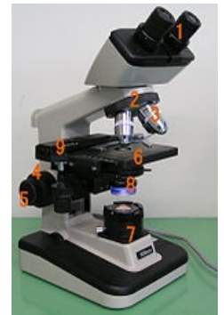
The main components of a light microscope: 1) eyepieces, 2) revolving turret, 3) objectives, 4) macroscrew, 5) microscrow, 6) stage, 7) light source, 8) condenser and diaphragm, 9) cross shift
