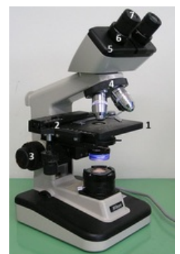
Mechanical system of an optical microscope: 1) stage, 2) cross shift, 3) macroscrew and microscrow, 4) revolver, 5) tube, 6) focusing ring, 7) eyepiece.
