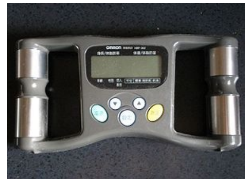
Device for measuring body fat % using bioelectrical impedance
